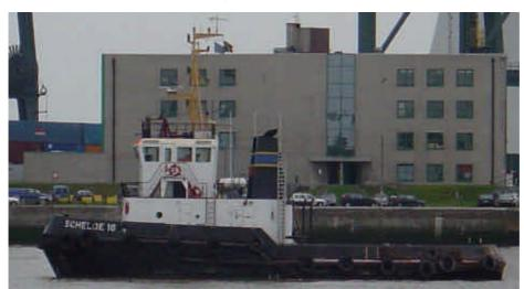
One of the older "conventional" tugs in the Port of Antwerp is the **SCHELDE 10**, this vessel is powered by two 'MWM' 6 cil. diesel engines totalling 1,800 kW at 1,000 rpm, driving two propellers in 'Kort' nozzles which give the vessel a maximum bollard pull of 32 tons.
