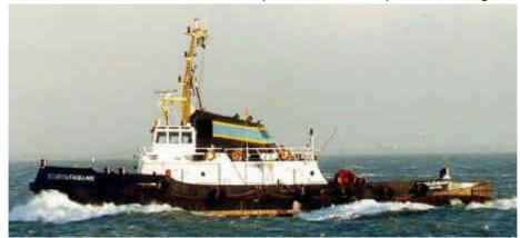
can be see at the picture (I don't know who made this photo), the SCHOUWENBANK measures 33 mtr in length and is powered by two 'Stork Werkspoor' type 6 FHD 24D 6 cyl. 1,300 kW medium speed diesel engines. Each engine drives a
