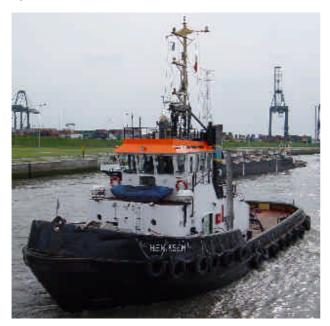
On deck the vessel is equipped with a Hydraulic towing winch combined with anchor windlass on forecastle deck and an identical towing winch, combined with bridle winch on aft deck. Towing winches: Brake holding: 80 -95 tons, dynamic: 28 tons at 26 m/ min, Slack rope speed: 50 m/min. Bridle winch: Brake holding: 53 tons - dynamic: 10 tons at 26 m/min. 45 tons SWL towing hook with 3
