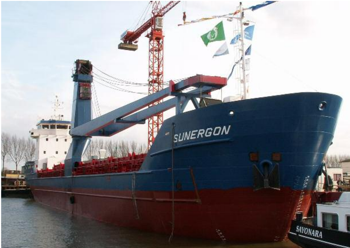
Seen in Werkendam the SUNERGON (Imo 9362580) owned by Gebr Trommel-Nijkerk , is measuring 89 x 12.5 mtr with a DWT of 3200 ton.
