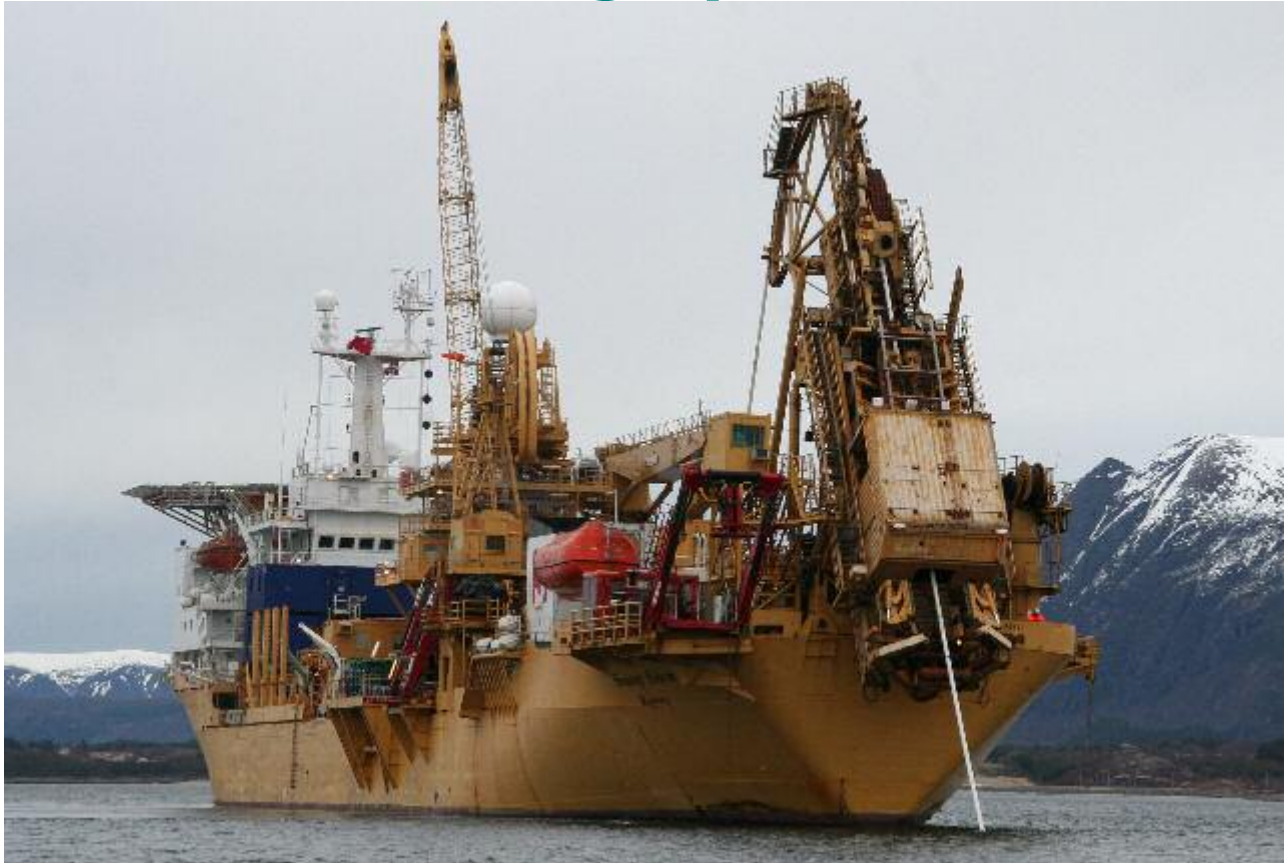
The SEAWAY FALCON seen laying the first 6" pipe for the Ormen Lange project, Photo : Jan Plug ©
