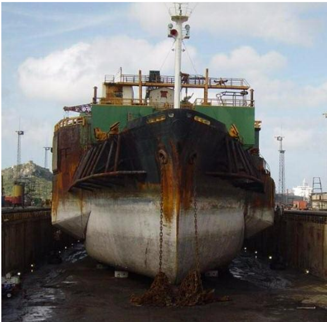
The PROTEXA/MEXICO owned HUASTECHO seen in the A-Dock at Curacao for approx. 800 ton steel renewal Photo : John Smit ©
