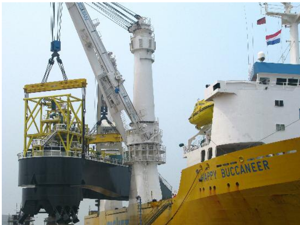
The HAPPY BUCCANEER seen loading the FSO Bunga Orkid turret at Penglai, China Photo : Capt. Jelle de Vries ©
