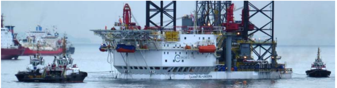
The AL JASSRA is a Baker Marine Services Pacific Class 400 rig which is built at the PPL Shipyard in Singapore for Gulf Drilling International
