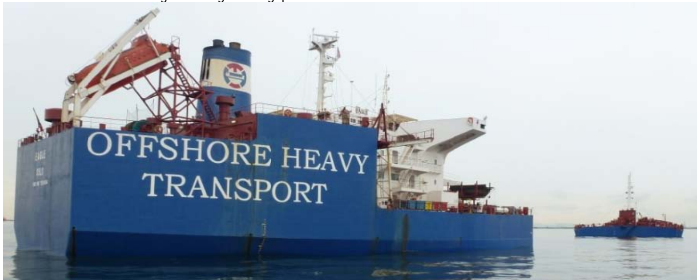
The EAGLE submerged to 17.5 mtr draft ready to load the AI JASSRA - Photo's : Piet Sinke ©
