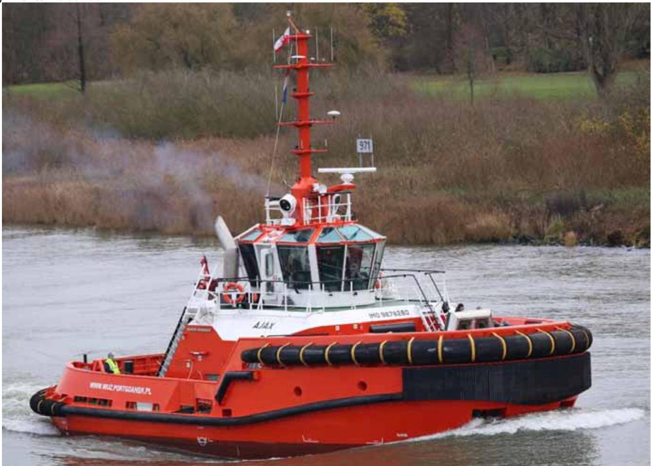
The Damen Build ASD tug 2312 AJAX passing Baanhoek bridge on river Merwede after yard period at Damen Hardinxveld where the AJAX is equipped with fully FIFI 1 system. Photo : Arie Boer (c)
