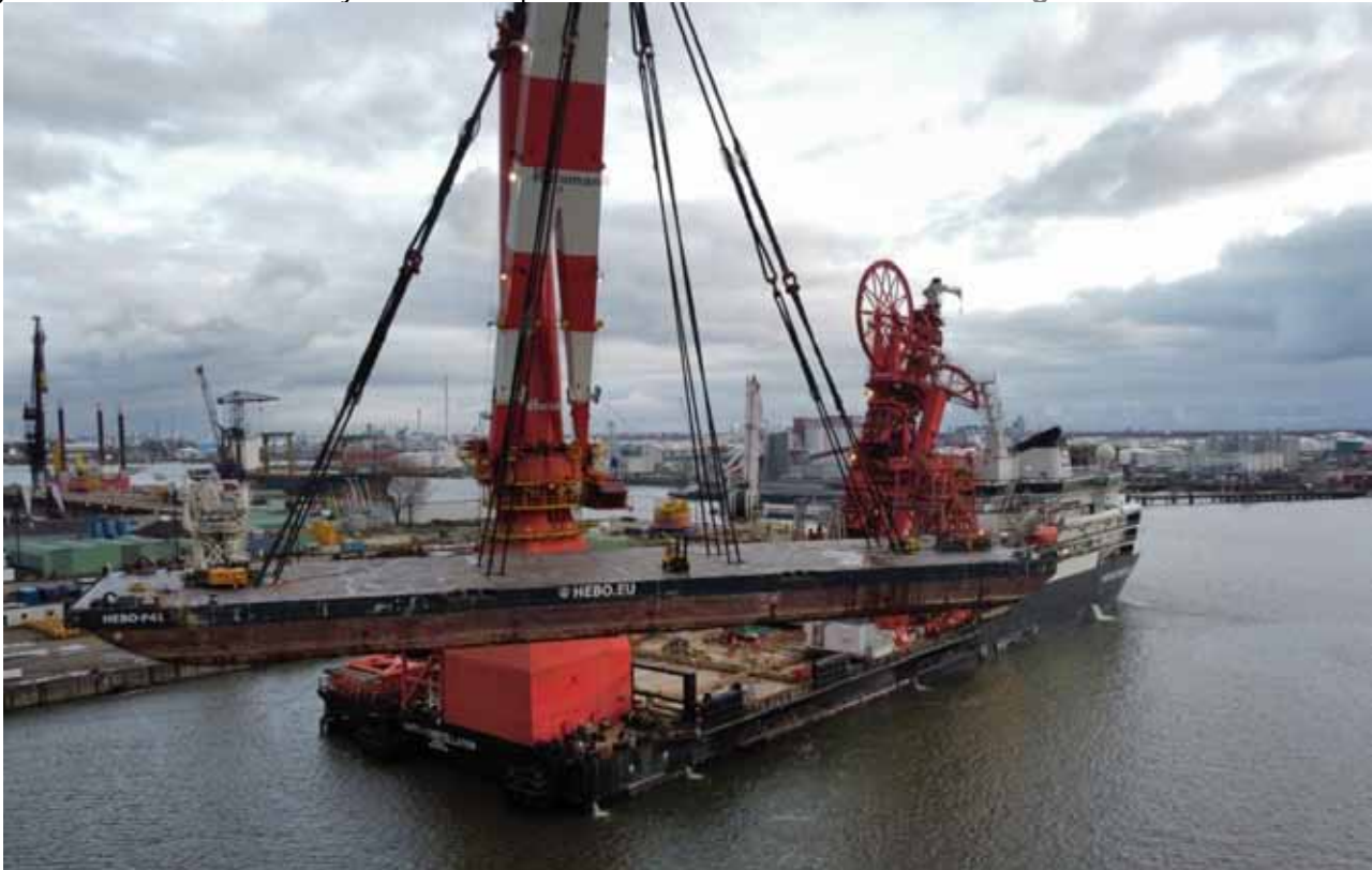
3300te Loadtest at the SAIPEM CONSTELLATION by HEBO maritime .
